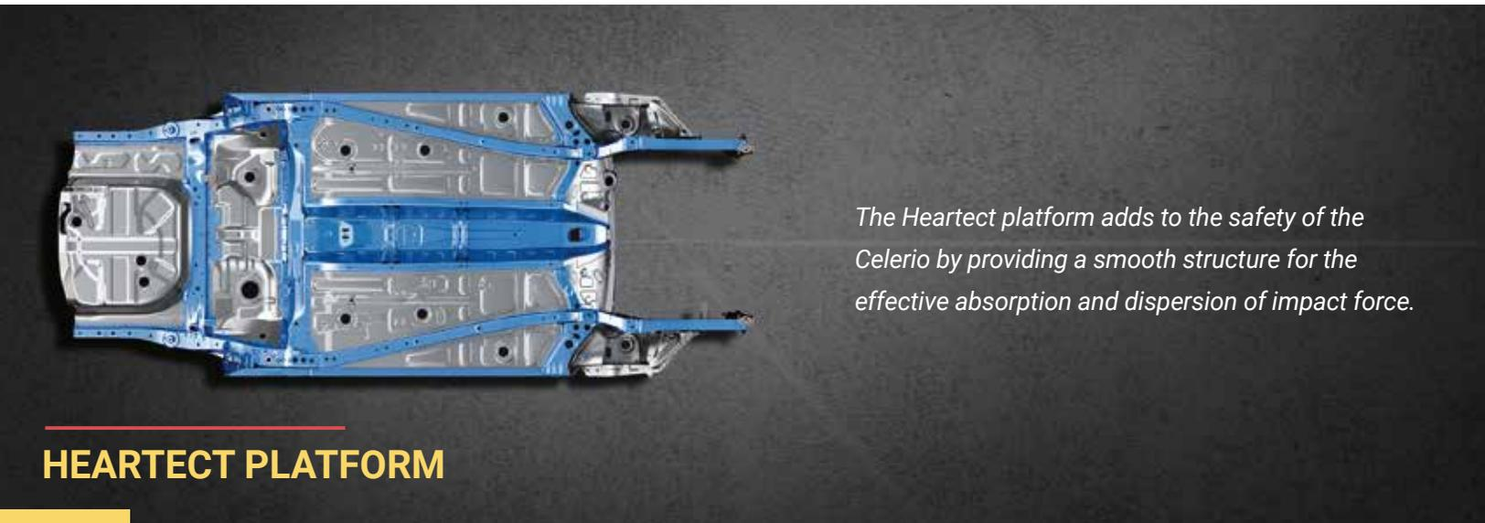
The Heartect platform adds to the safety of the Celerio by providing a smooth structure for the effective absorption and dispersion of impact force.
